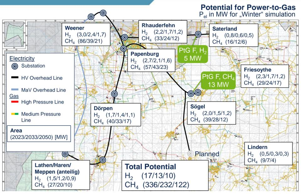
The necessary electricity intake for the PtG facilities (5 MW H<sub>2</sub>, 13 MW CH<sub>4</sub>) could be achieved through redirection of gas in the gas network.
