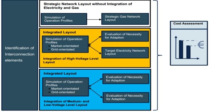
Evaluation of the separate and integrated planning of electricity and gas networks through cost comparison.
