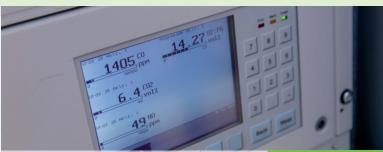
Measured value display exhaust gas analyser
