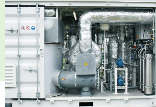
Reformer for the production of 100 m 3 (i.N.)/h H 2
