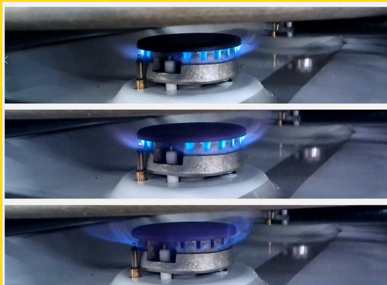
Flame with partial flash back on a cooker hob (picture THyGA test DGC)
