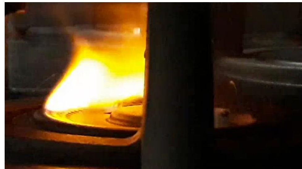
EN12 burner under normal operation and with water falling into the flame
