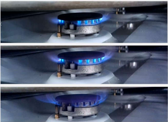
Test showing FB under following test conditions, Q_{max} , P_{nom} , CH_4 = 40\% H_2 = 60\%
