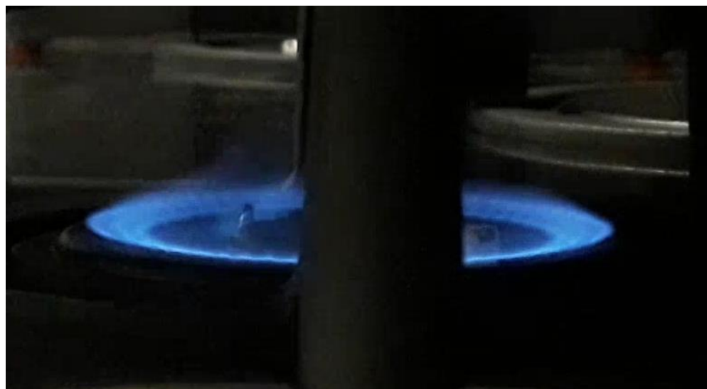
EN12 burner under normal operation and with water falling into the flame
