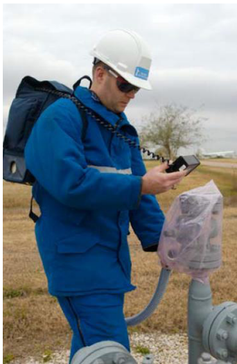
Figure 5: High Flow Sampler Measurement on a Facility
