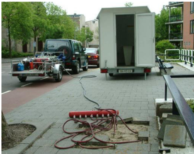
Figure A.2: Emission Rate Measurement with Suction Method in Amsterdam
