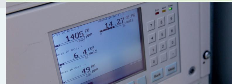
Measured value display exhaust gas analyser
